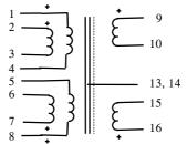
**Spacing between pins:** 2.54 mm (0.1") **Spacing between rows of pins:** 22.86 mm (0.9") 30 g
