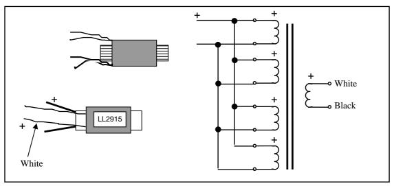
Weight: Core: Static resistance of primary: Static resistance of secondary: 34 g Mu metal lamination core 0.05  $\Omega$  69  $\Omega$
