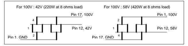
Static resistance, pin 1 to pin 17: Static resistance, pin 1 to pin 12: Max signal voltage, pin 1 to pin 17 at 50 Hz: Transformer no load impedance, pin 1 to pin 17 at 100V, 50Hz 1.2 Ω
